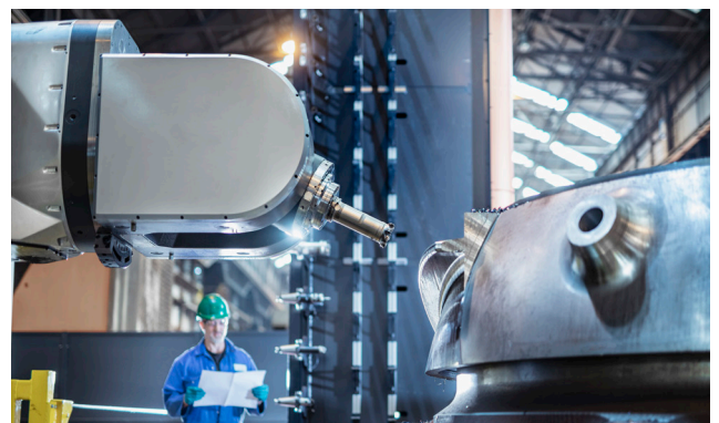
5-Axis Machining of an Ultra-Large Component
