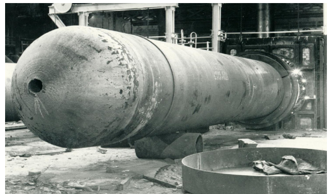
A boiler drum being forged at Brightside Lane
